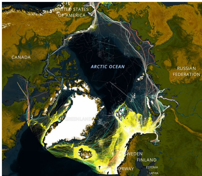
Map 7. Ship traffic lines in the Arctic in 2012 (north of 60°N). The ship traffic observations are made through the satellite-based Automatic Identification System (AIS), which provides the identification of the spatial location of a vessel at a given time. Ship tracks denote the estimated routes undertaken by ships. Data-source: Automatic System (AIS) data, provided by The Norwegian Coastal Administration / www.havbase.no (2013) and further processed by DNV and WWF. http://wwfarcticmaps.org/DIQAB7
